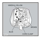
The wire coloured green and yellow must be connected to the terminal marked with the letter «E» or by the earth symbol  $\sqsubseteq$  or coloured green and yellow.
